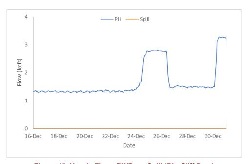
Figure 15. Hourly Flows PWR vs. Spill (Big Cliff Dam)
